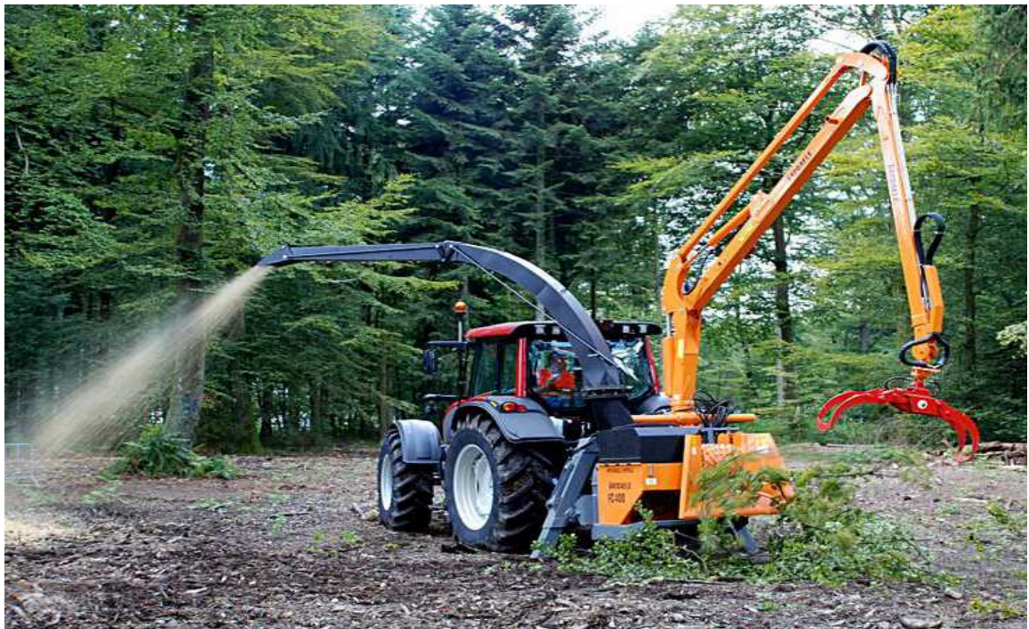
Illustration 6: Tractor PTO powered chipper with feeding attachment
